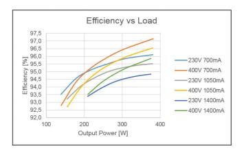
Typical Efficiency vs. Load OT FIT 380/220-400/1A4 D NFC HCL
